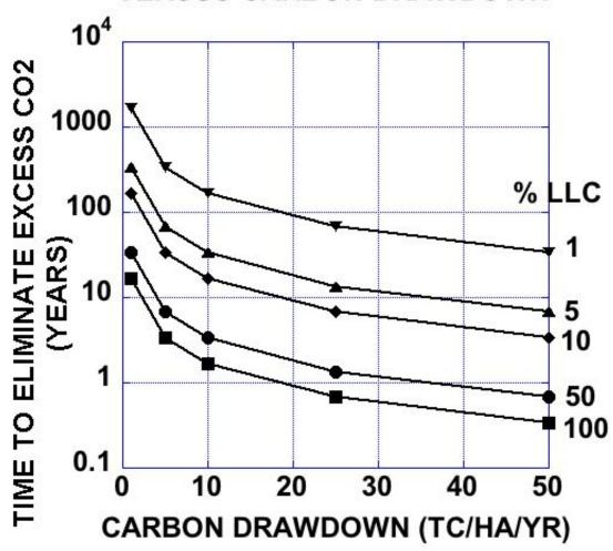
FIGURE 2. Time to eliminate dangerous excess carbon versus rate of carbon drawdown for various percentages of long lived carbon (Goreau, 2016)
