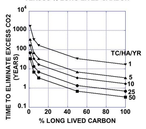
FIGURE 3. Time to eliminate dangerous excess carbon versus percentages of long lived carbon for various rates of carbon drawdown (Goreau, 2016)
